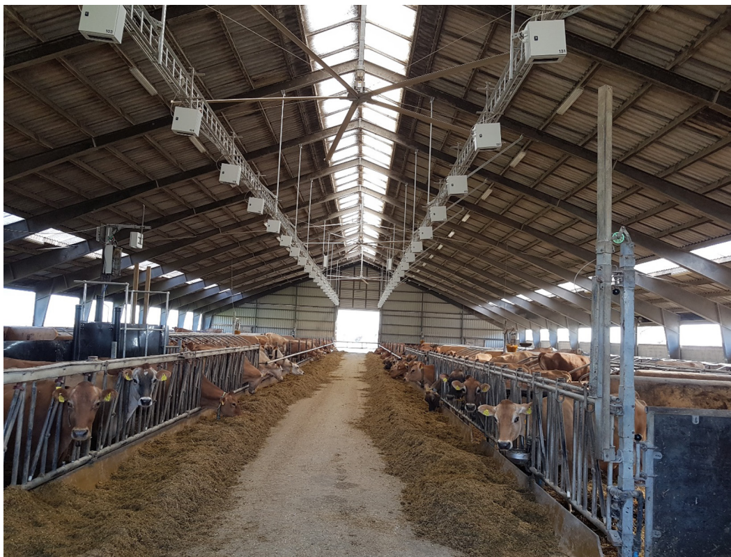
Figure 1. Example of setup of the Cattle Feed Intake System. The cameras are placed 4.5 m in the air, 2.3 m apart. The passage box in the left part of the barn is used for reading ear tags and taking simultaneous image for BW prediction and identification at the feeding table.
